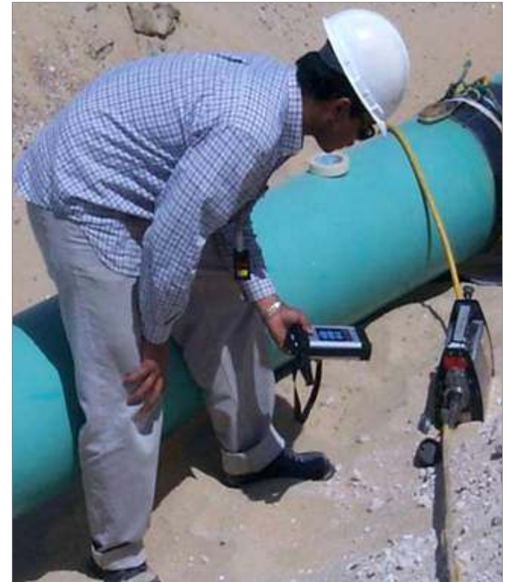
Industrial radiography of pipes using Iridium-192
